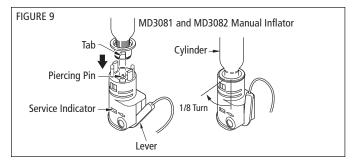
5) Examine the service indicator (Fig. 9) and ensure it is GREEN. If the service indicator is red, the mechanism has been fired or is incorrectly fitted and the inflator requires service. See Re-arming Your PFD (MD3081 and MD3082) p. 8.
